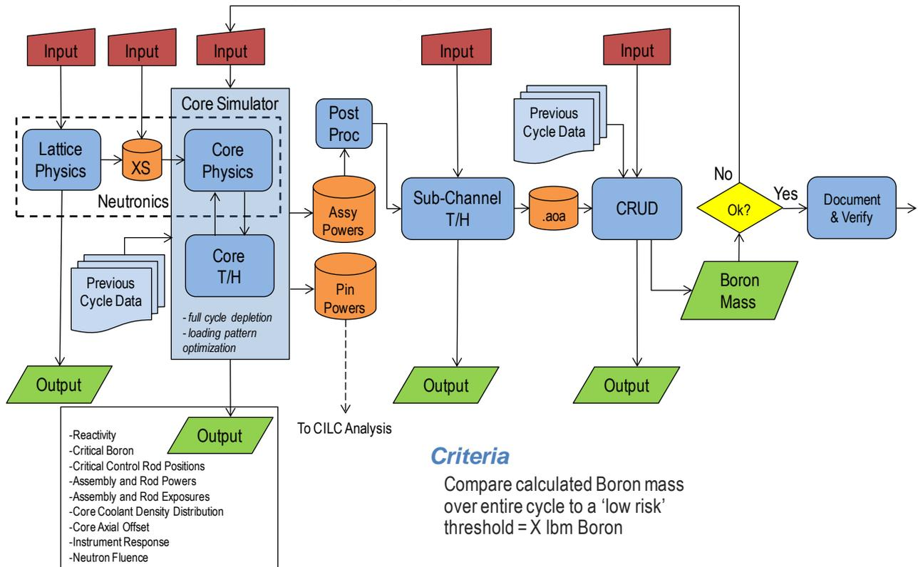
1. The reactor core neutronics simulations are supported by macroscopic cross section libraries that are generated prior to performing this analysis. This data is provided by a 2D lattice physics code, as described in the previous discussion on the core simulation workflow.
