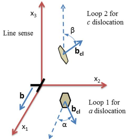
Fig. A1. Orientation of prismatic loops near dislocation line.
