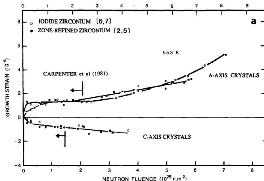
**Fig. 3.** Dose dependence of growth strain in neutron-irradiated pre-annealed single Zr crystals (from [23]). Note that the absolute values of the  $c$  strain are smaller than that in  $a$  direction.
