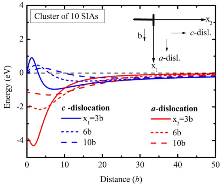
Fig. A2. Interaction energy of a 10 SIA cluster with  $a$  and  $c$  dislocations calculated using Eq. (A2). The red curves correspond to the case  $\alpha = 0$ , the blue ones to  $\beta = \pi/2$ .
