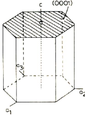
**Fig. 4.** Main crystallographic directions in hcp crystals.
