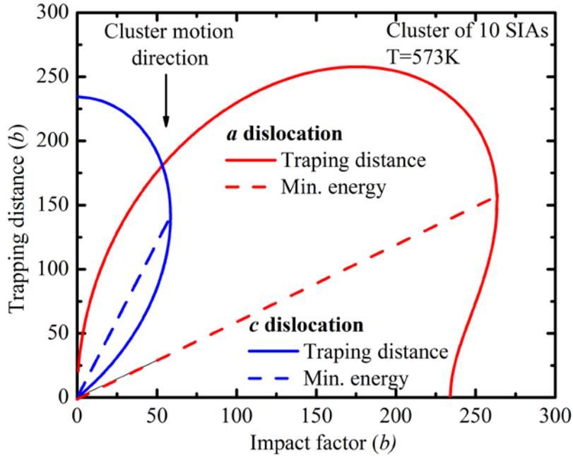
Fig. A3. Trapping zones of  $a$  and  $c$  dislocations for a cluster of 10 SIAs.
