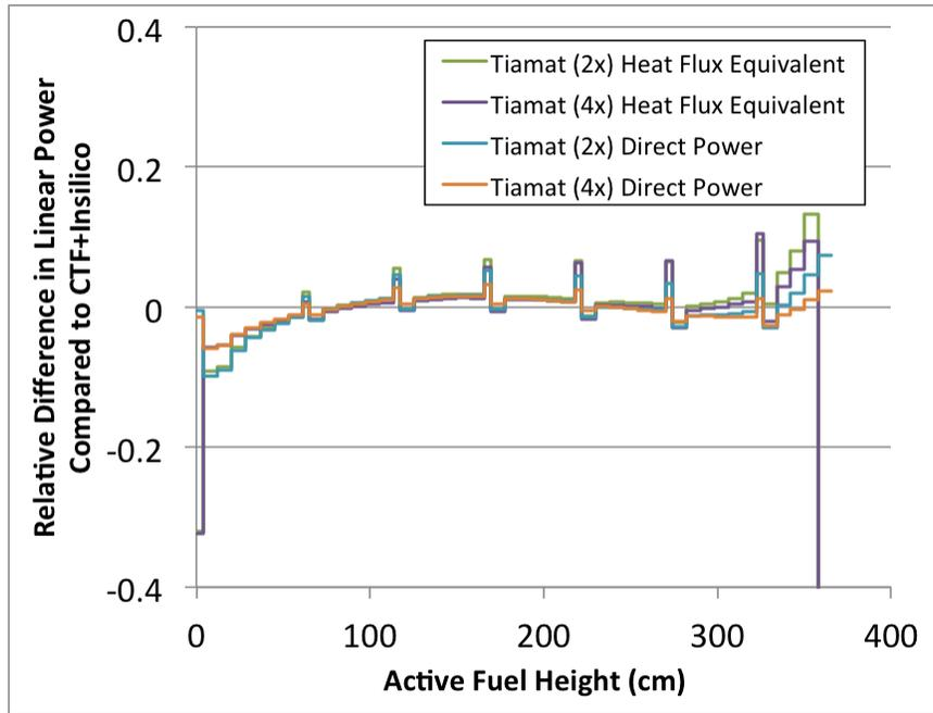
**Figure 3. Power shape of CTF+Insilico and Tiamat for mesh refinement with CTF heat flux equivalent power.**
