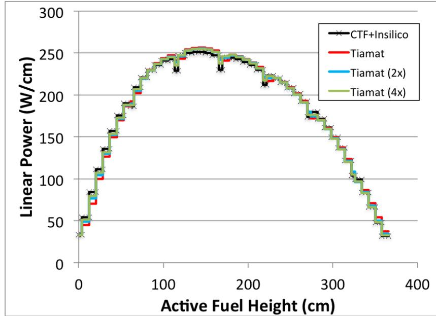
**Figure 2. Axial Power Shape of CTF+Insilico and Tiamat with Mesh Refinement**
