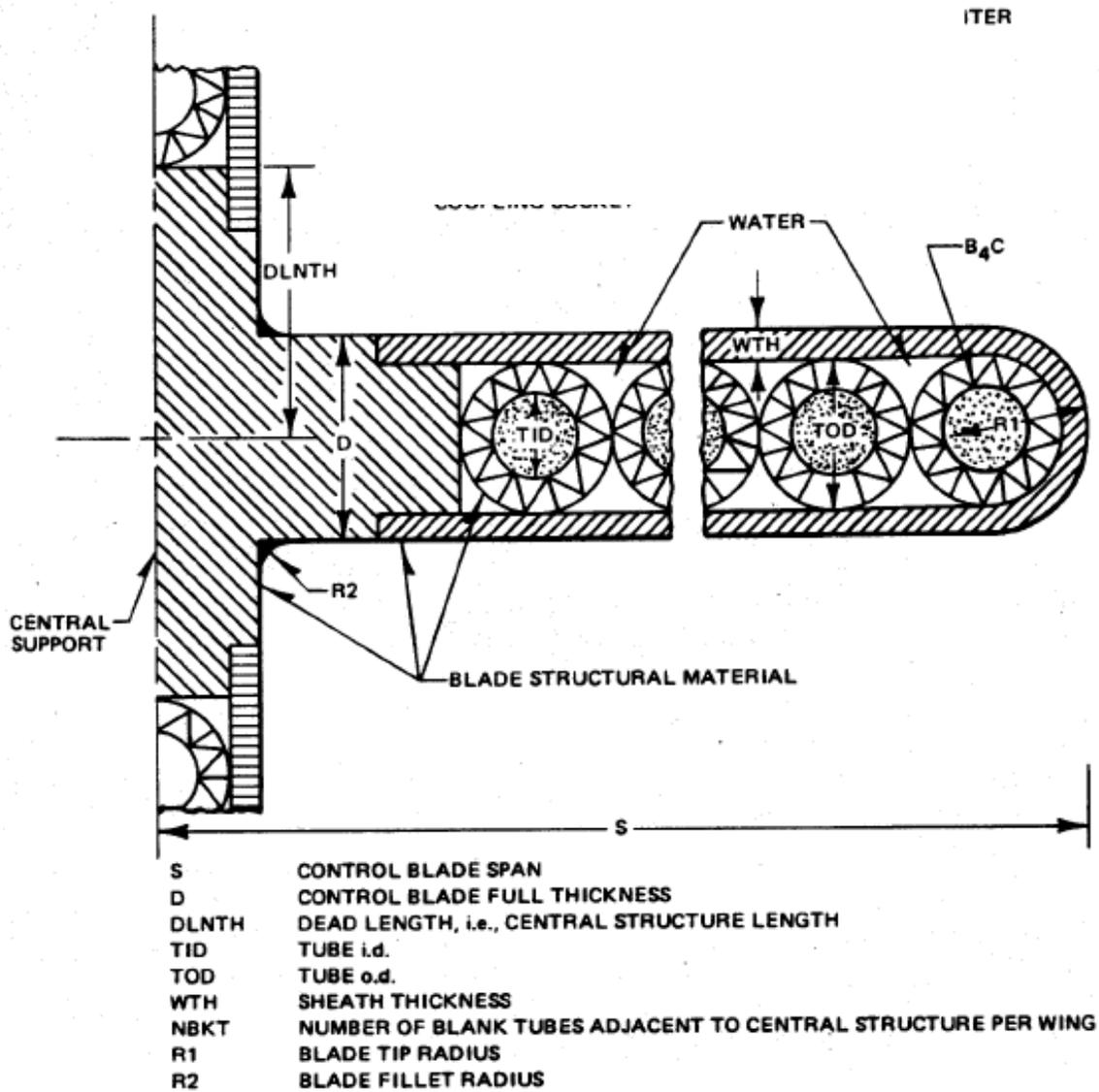
Figure 3: Control Blade Geometry [3]
