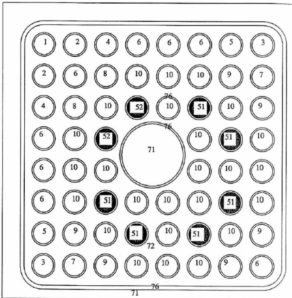
Figure 2: Material Composition for GE9 Assembly. The solid rods are gad rods [1].
