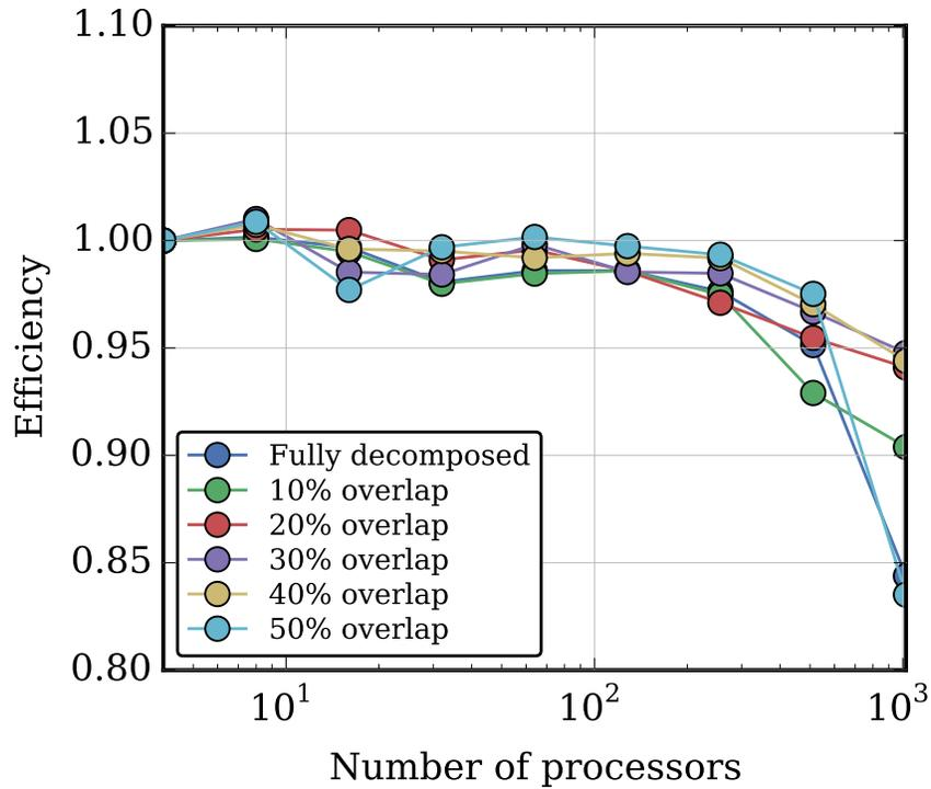
**Figure 4. Strong scaling plot of the 4x4 reactor assembly problem on Titan showing efficiency versus the number of sets. Each set is decomposed into 2 x 2 blocks.**
