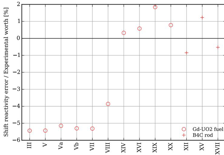
**Figure 2. Absolute error of Shift simulations of Gd-UO<sub>2</sub> fuel and B<sub>4</sub>C rod worths from the BW1810 experiment.**
