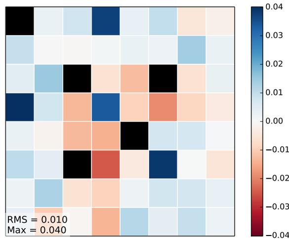
**Figure 1. BW1810 core-XIV relative difference in midplane pin powers for a quarter of the center assembly at the midplane between Shift and the benchmark.**
