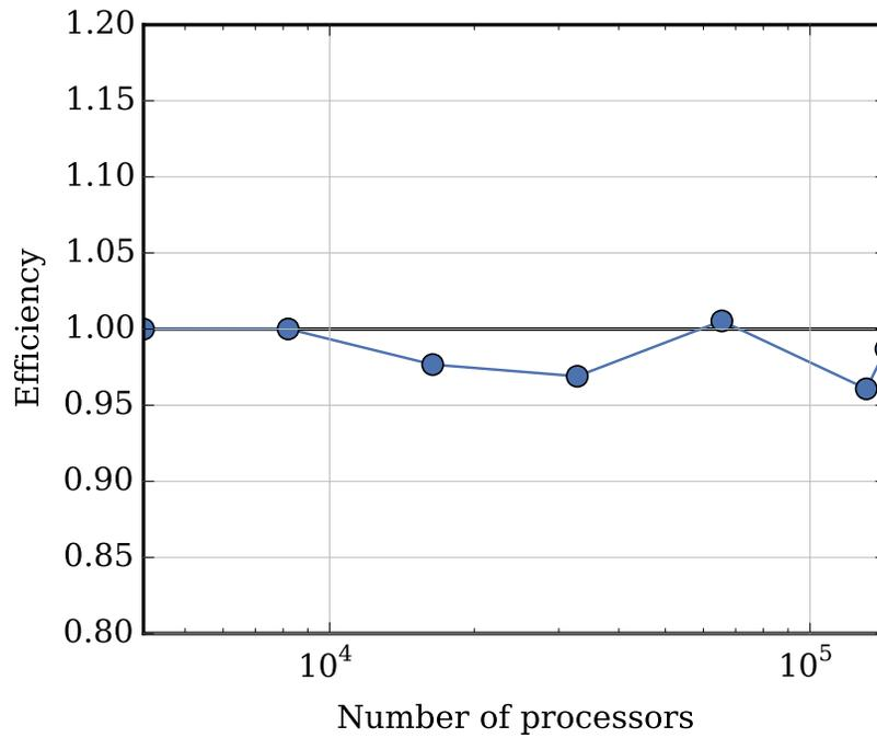
**Figure 3. Shift strong scaling results for AP1000® problem 1 on Titan.**
