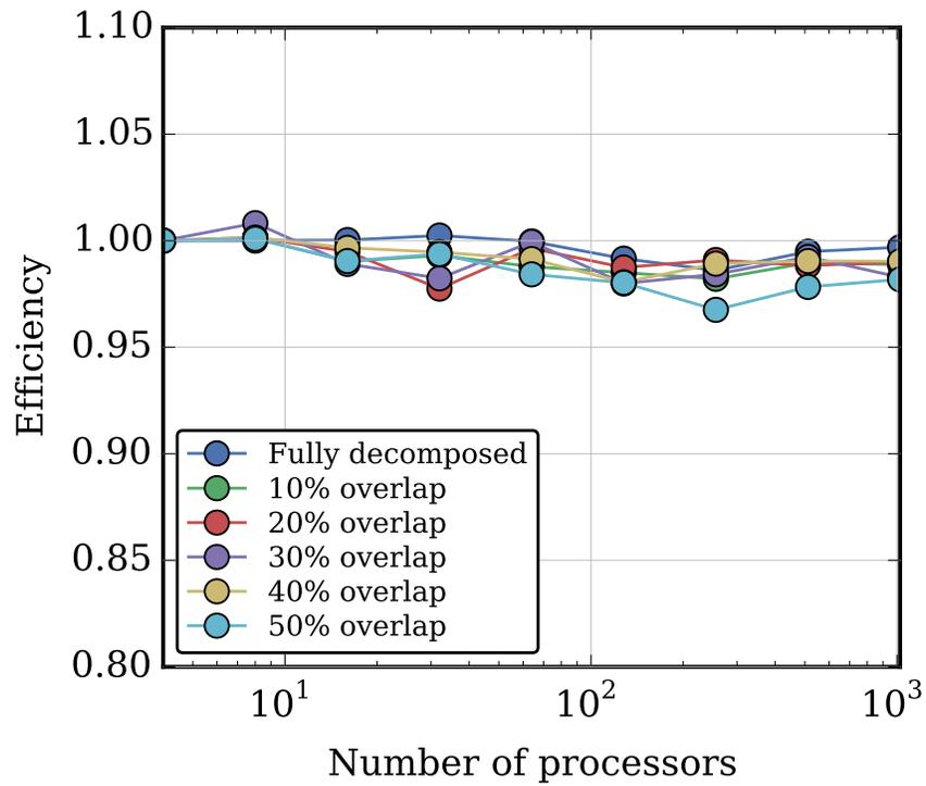
**Figure 5. Weak scaling of the  $4 \times 4$  reactor assembly problem on Titan with each set decomposed into  $2 \times 2$  blocks. This plot shows efficiency versus number of sets. The multi-set solve time is normalized by the single-set solve time to produce these efficiency results.**
