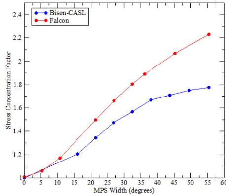
Figure 13. 2-D Stress concentration factor, as a function of MPS defect width compared to values from the literature [3].
