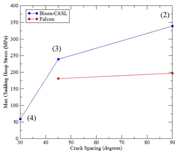
**Figure 7.** The maximum clad hoop stress calculated in a 2-D (R-Theta), 90 degree model as a function of the number of radial cracks.
