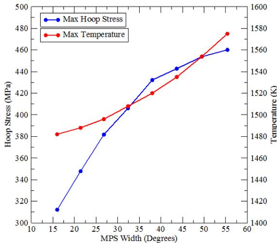
**Figure 12.** 2-D Bison-CASL calculations of a 180 degree pellet containing 3 radial cracks of 70% length, and a MPS, which shows the affect of increasing the MPS width on the maximum clad hoop stress (blue curve) and maximum fuel centerline temperature (red curve).
