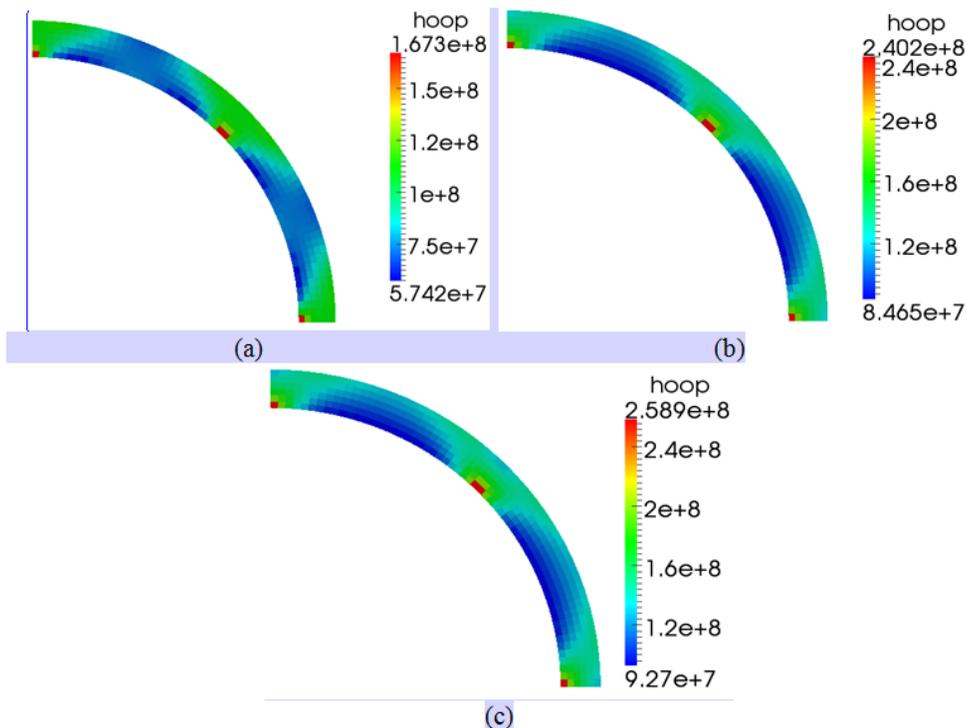
Figure 9. (a) Hoop stress contour plot for the 30% radial crack model, (b) Hoop stress contour plot for the 50% radial crack model, and (c) Hoop stress contour plot for the 70% radial crack model.
