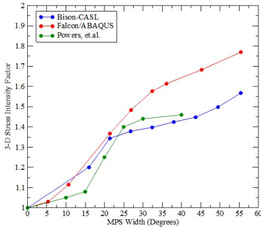
**Figure 19.** 3-D Bison-CASL stress concentration factor, as a function of MPS defect width, compared to values from literature [3,13].
