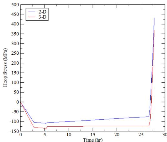
**Figure 17.** Comparison of the hoop stress calculations a 2-D R-Theta 180 degree model MPS with a width of 105 mil (blue line) to a 3-D 180-degree model containing a MPS of width 105 mils and length of 105 mils (red line).
