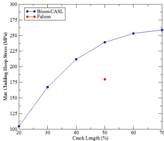
**Figure 8,** 2-D Bison-CASL R-Theta calculations of a 90-degree pellet containing 3 radial cracks showing the influence of crack length on the maximum clad hoop stress.
