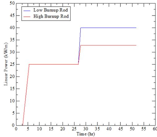
Figure 6. Power histories used to simulate the impact of discrete cracks and MPS on the local cladding hoop stress.
