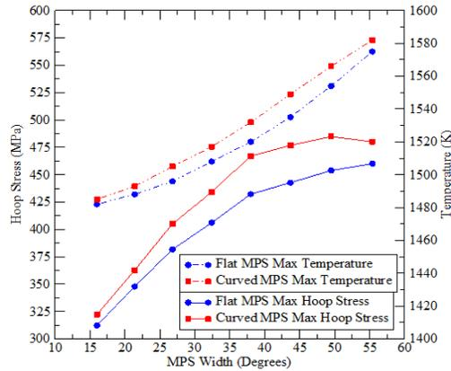
**Figure 14.** Cladding Stresses Calculated by Bison-CASL for Various Size MPS Defects, along with the Corresponding Maximum Temperature in the Fuel Pellet.
