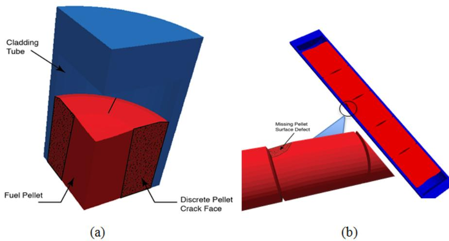
**Figure 5.** (a) 3-D geometric representation of a cracked pellet., and (b) 3-D geometric representation of a 5-pellet rodlet with the center pellet having an MPS defect.
