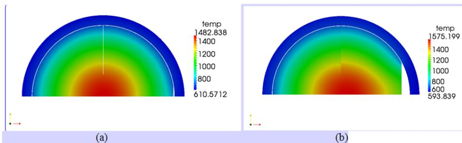
Figure 11. (a) Temperature Contour at Peak Cladding Stress Time for a 45-mil Flat MPS Defect, and (b) Temperature Contour at Peak Cladding Stress Time for a 150-mil Flat MPS Defect.
