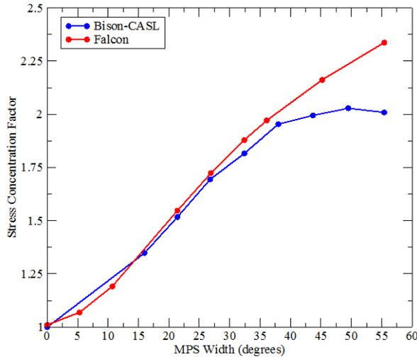
Figure 15. 2-D Stress concentration factor using the same geometric models, e.g. crack length, MPS shape, and 90 degree model, as a function of MPS defect width compared to values from the literature [3].
