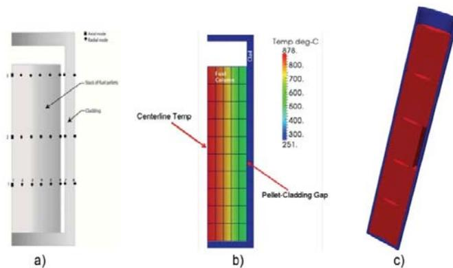
**Figure 2.** 1/1.5D-2D R-Z (a) 1/1.5-D Geometric Representation, (b) Falcon or Bison-CASL 2-D R-Z Fuel Rod Representation, and (c) 3-D Bison-CASL 5-Pellet Model Containing a MPS and the Cladding [16].
