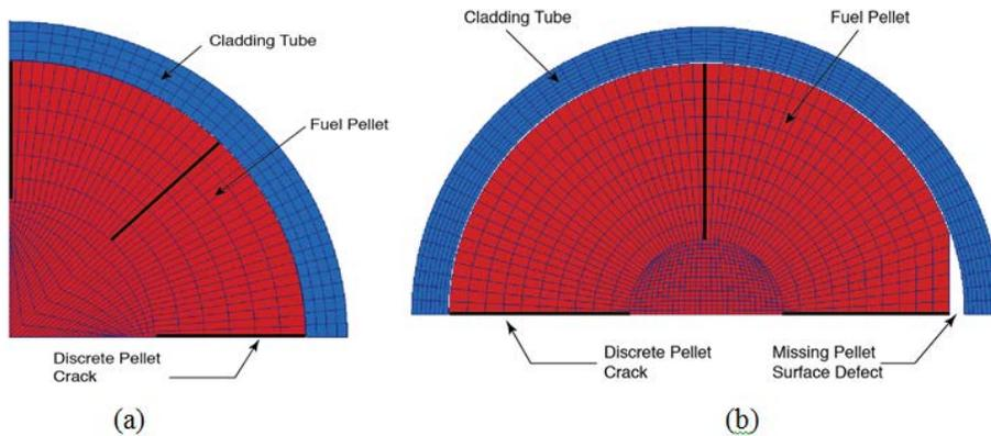
**Figure 4.** (a) 2-D, R-Theta model showing a representative three crack geometry (at 0, 45 and 90°, respectively) of radially oriented half-length cracks in the fuel pellet, and (b) Geometric representation of an MPS defect in 2-D R-Theta space.
