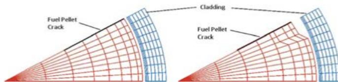
**Figure 3.** Falcon representation of a fuel pellet and cladding containing a crack and a MPS in the fuel in R-Theta space, as reproduced from Reference [16].
