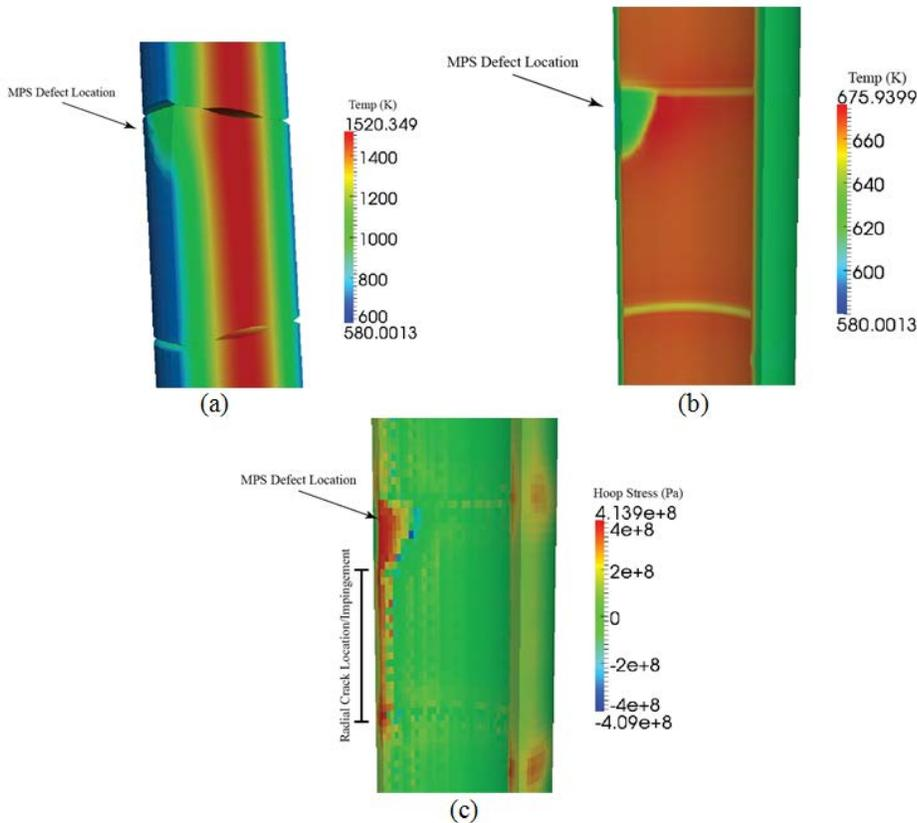
**Figure 18.** (a) Pellet temperature distribution in the vicinity of the MPS defect, (b) Inner cladding surface temperature distribution in the vicinity of the MPS defect, and (c) Inner cladding surface hoop stress distribution in the vicinity of the MPS defect.
