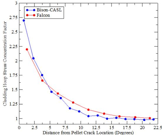
**Figure 10.** Clad hoop stress concentration factor as a function of the angular position from the fuel pellet crack location for a 70% long radial crack in a 2-D, R-Theta geometry.
