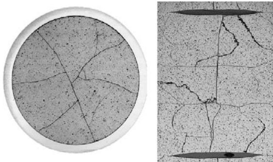
**Figure 1.** Fuel pellets irradiated under normal operating conditions (specify these --- burnup, max linear power, etc), as reproduced from Ref [15].
