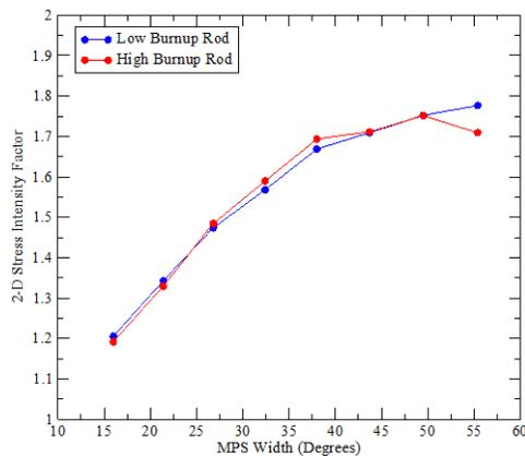
Figure 16. Comparison of 2-D Stress concentration factor for a low burnup rod and a high burnup rod, as a function of MPS defect width.
