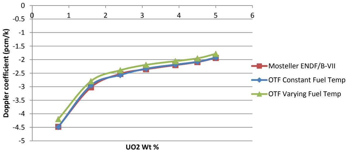
**Figure 3. Doppler Reactivity Defect for UO<sub>2</sub> Benchmark Cases**
