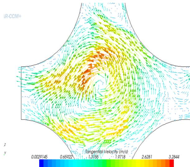
Figure 6 (b) Lateral velocity vectors from CFD at 1.97 inch above grid strap
