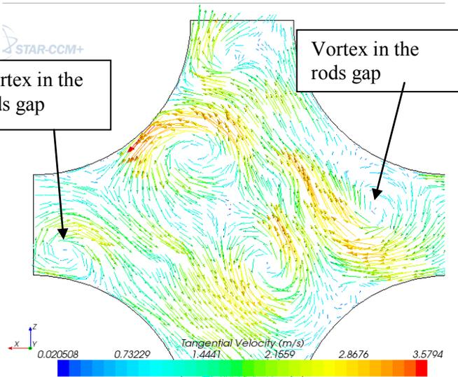
Figure 5 (b): Lateral velocity vectors from CFD at 0.67 inch above strap
